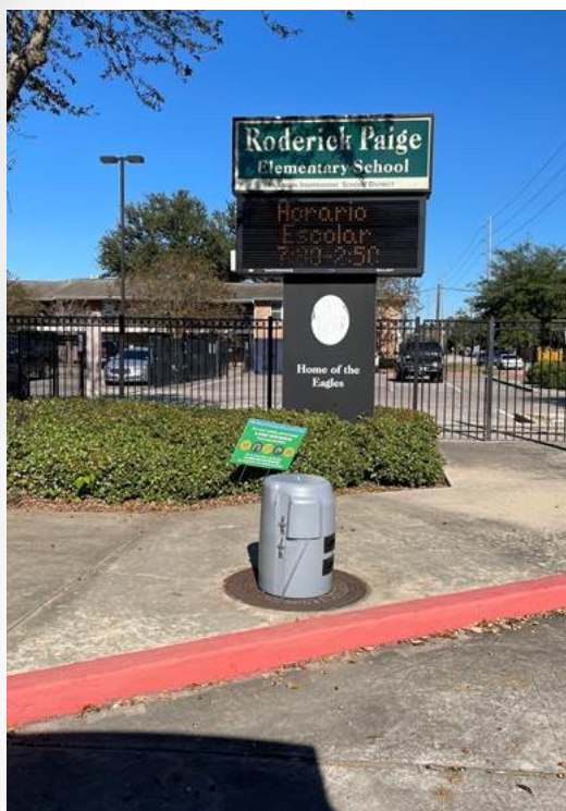
Figure 2. HACH AS950 portable automatic water sampler installed at elementary school
