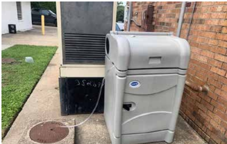
Figure 1. HACH AS950 all-weather, refrigerated automatic water sampler installed at nursing home
